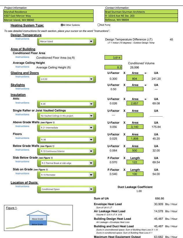
Building and Duct Heat Loss X 1.40 for Forced Air Furnace Building and Duct Heat Loss X 1.25 for Heat Pump
