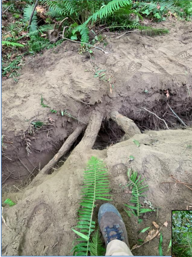
Photo # 4: Looking down at the only Douglas Fir tree roots encountered from the two subject trees. A fourth root was encountered at the bottom of the trench at approximately 30 inches of depth. They measured 2.9", 4.6", 3.7", & an estimated 2.5".
