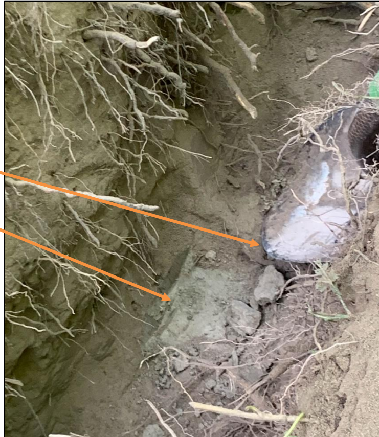
Photo # 3: Looking down into the trench. At approximately 26 to 34 inches below the surface solid blue clay was encountered. In a few random places the operators forced their way into the clay to a depth of 44 to 46 inches. They encountered solid clay at those depths also.
