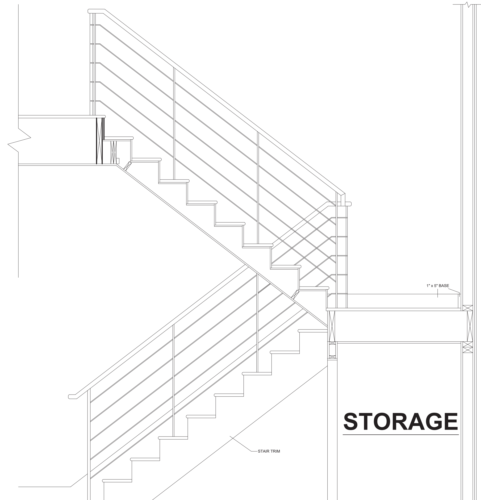
STAIRCASE SECTION NTS
