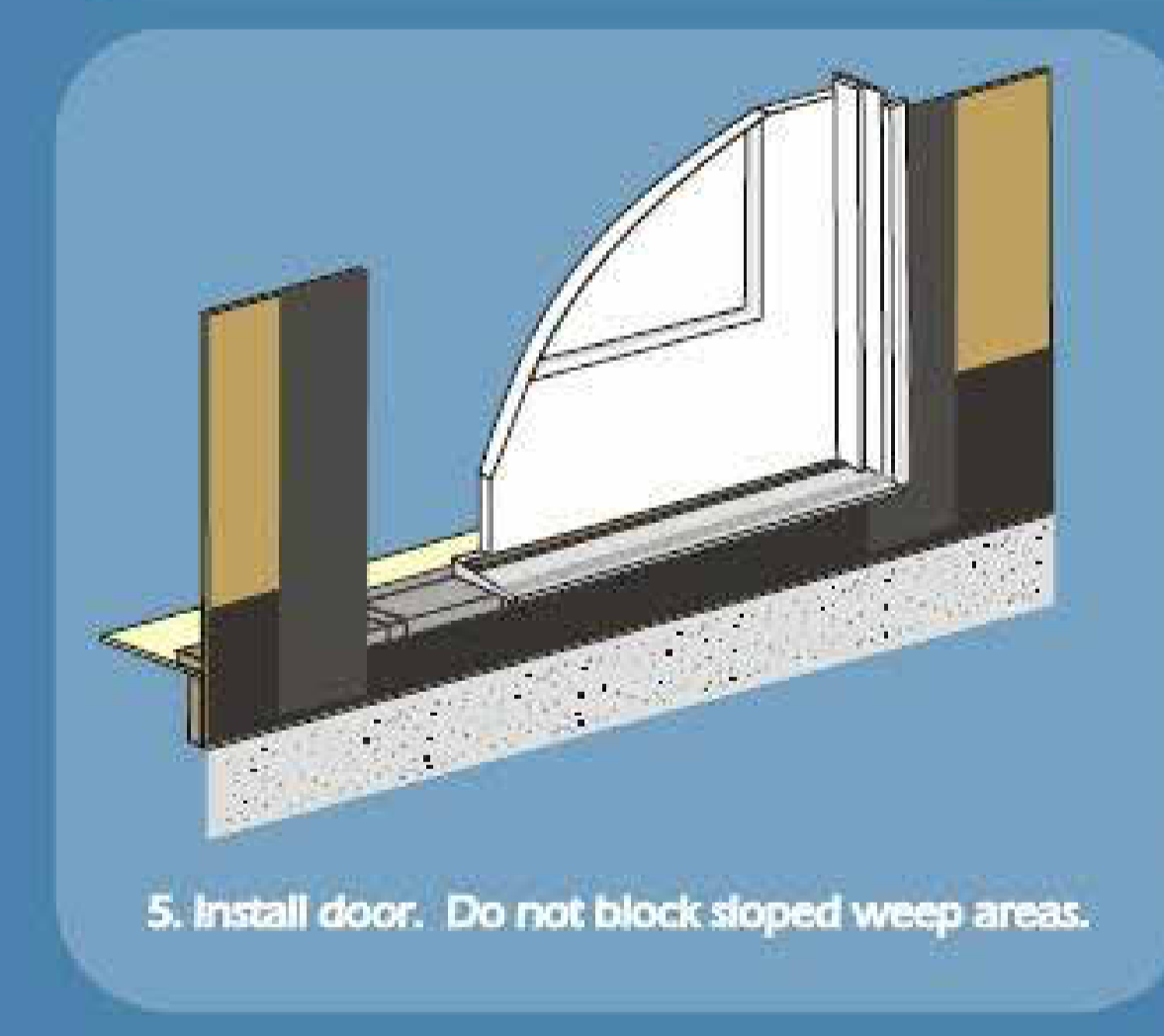
2 DOOR FLASHING A505.1 1/2" = 1'-0"
