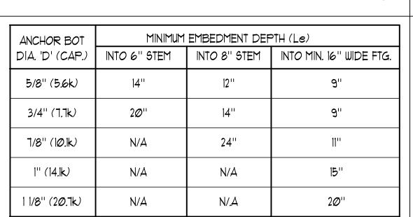
HOLDOWN EMBEDMENTS LISTED ARE BASED ON THE ALLOWABLE CAPACITIES DEVELOPED IN CONCRETE WALLS WITH TYPICAL REINFORCING SPACED NOT MORE THAN 18" ON CENTER.
