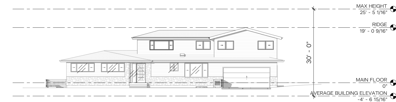
4 NORTH ELEVATION - MAX BUILDING HEIGHT 1/16" = 1'-0"
