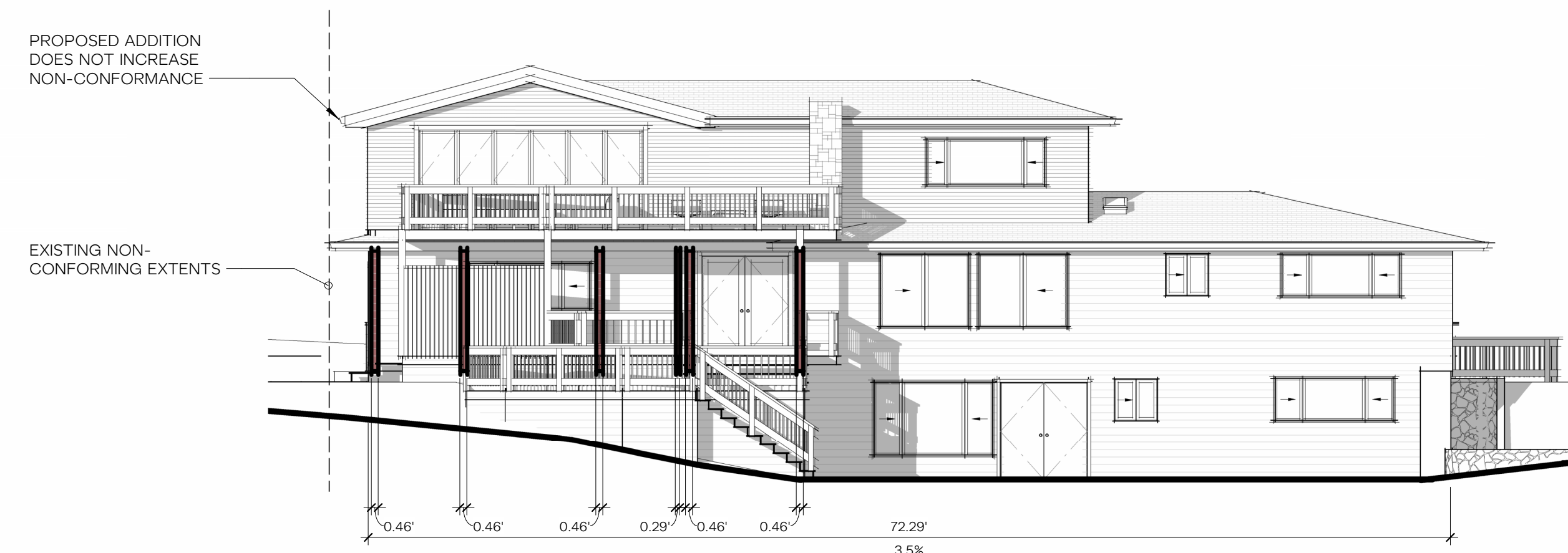
1 SOUTH ELEVATION - NON-CONFORMING STRUCTURE
