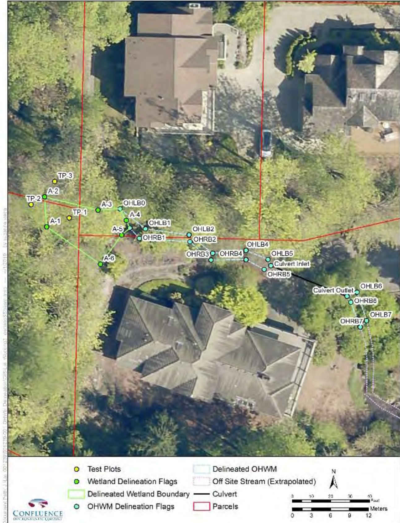
Figure 2. Location of Test Plots and Critical Area Boundaries
