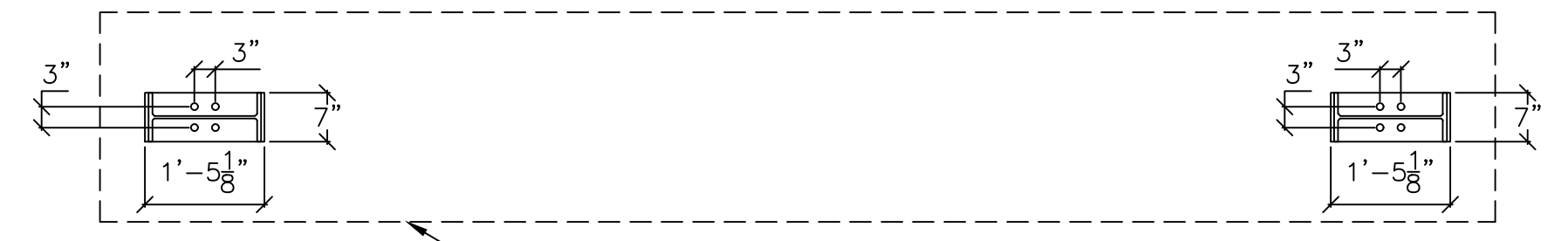
GRADE BEAM PER DESIGNER FRAME MODEL: SMF16z16-151.75x220.375-(MF4-3)
